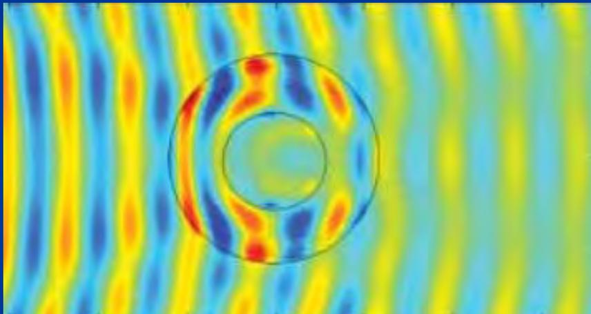
D. Schurig, *et al.* Metamaterial Electromagnetic Cloak at Microwave Frequencies *Science* 314, 977 (2006);
